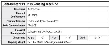
NOTE: Models with coils can be easily changed as required for vending different size products. Coils and dividers as well as individual tray price scrolls are available from our parts division Vendnet for an additional cost.
